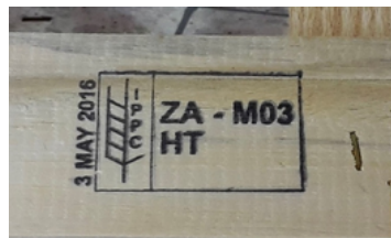
ISPM 15 mark on WPM © T. Schroeder, BMEL, Germany
